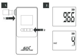
Insert the mouthpiece into the measurement port (\*1). Turn on the device by pressing the function button on the main panel (\*2).
