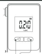
The breathalyzer is ready to take a measurement (\*1). Blow continuously for about 6 seconds. During the measurement, the breathalyzer will display the progress of the sample collection (\*2), and will signal the end with a short beep. After analyzing the sample, the breathalyzer will display the result (\*3). At this point, you can either wait 30 seconds for the breathalyzer to turn off automatically or press one of the buttons to perform one of the following actions:
