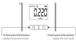
Holding the button for about 3 seconds: start the measurement. Holding the button for • about 3 seconds: turn off the breathalyzer.
