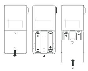
Press the battery compartment cover and slide it down (\*1). Slide the battery cover along the guides until it is completely detached. Then, place two 1.5V AAA (LR03) alkaline batteries in the battery compartment, ensuring correct polarity (see image) (\*2). After placing the batteries in the power compartment, align the battery cover with the device guides and slide it upwards until you hear a dick (\*3).
